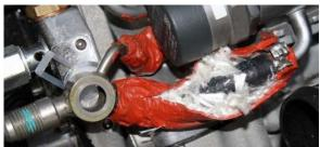
It is possible to cut the Injector Return Line [2] for an easier disassembly.
